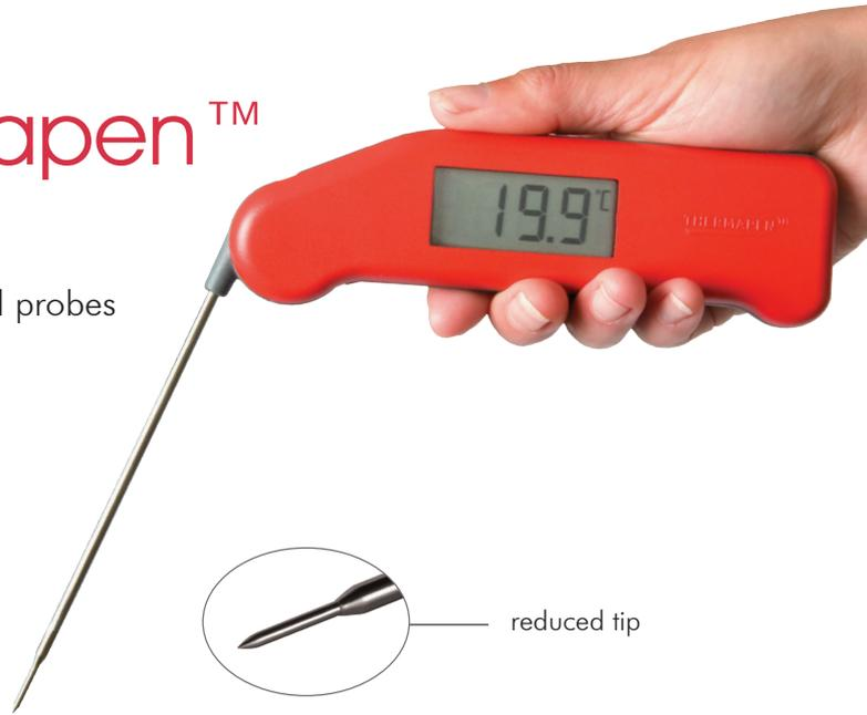
The SuperFast Thermapen thermometer incorporates a large digital display with a precise read-out of temperature over the range of -49.9 to 299.9 °C with a 0.1 °C resolution and an accuracy of ±0.4 °C. The resolution can be switched to 1 °C, if required, via a switch in the battery compartment. The thermometer will power off automatically after ten minutes, maximising battery life. This feature can be disabled if not required.
