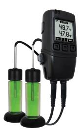
This standalone data logger measures and stores over 250,000 temperature readings over a -40 to +60°C (-40 to +140°F) range at a resolution of 0.1°C (0.2°F).
