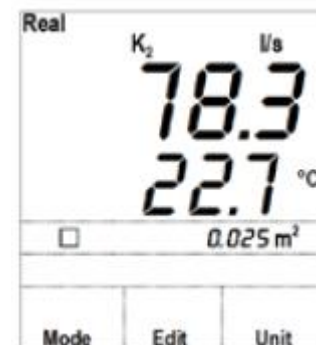
Air flow measuring with given transversal area
