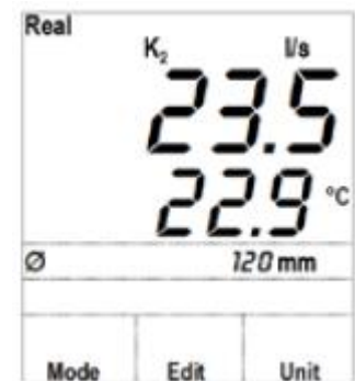
Air flow measuring with given diameter
