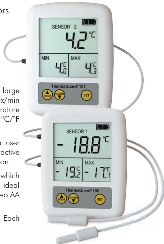
These high accuracy fridge or freezer thermometers feature a large LCD display, which simultaneously display the current and max/min recorded temperatures. The ThermaGuard measures temperature over the range of -39.9 to 49.9 °C (external sensor) with 0.1 °C/°F (switchable) with an accuracy of  $\pm 0.4$  °C.
