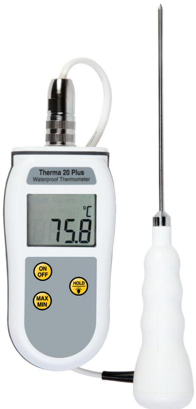
**INSTRUMENT OPERATION** - Where applicable (Therma 20 Plus and Therma 22 Plus) connect a probe via the socket located at the top of the instrument, screw in the collar of the plug, finger tight, to ensure a secure connection (do not over tighten). Switch the instrument on and apply the tip of the probe to the substance or medium to be measured. The instrument reading may take a few seconds to stabilise, depending on the nature of the measurement and sensitivity of the probe.
